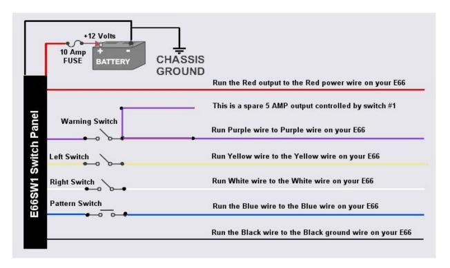
The Switch E66SW1 is designed to work specifically with the E66 series lightstick purchased after May 1<sup>st</sup> 2011. This switch features 6 outputs with quick splices on them allowing you to quickly wire your switch to your E66 series lightstick. We have also included an additional lead off the Warning Switch that will allow you to run other lights off the same switch. This lead is rated for 5 amps.
